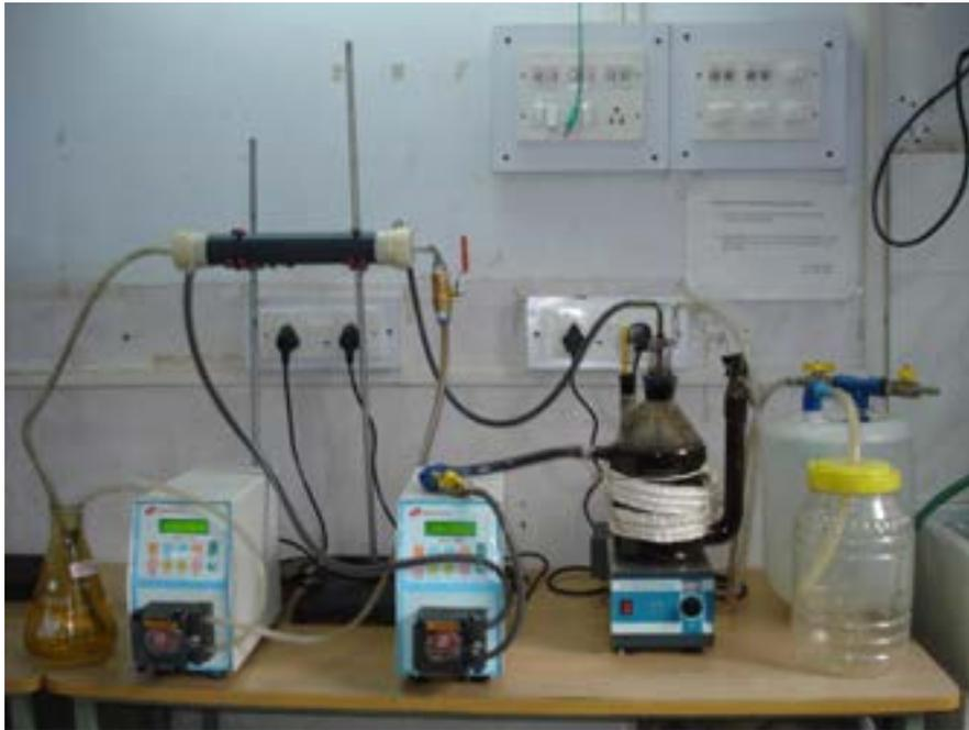
**EXPERIMENTAL SETUP FOR CONTINUOUS GAS GENERATION**
