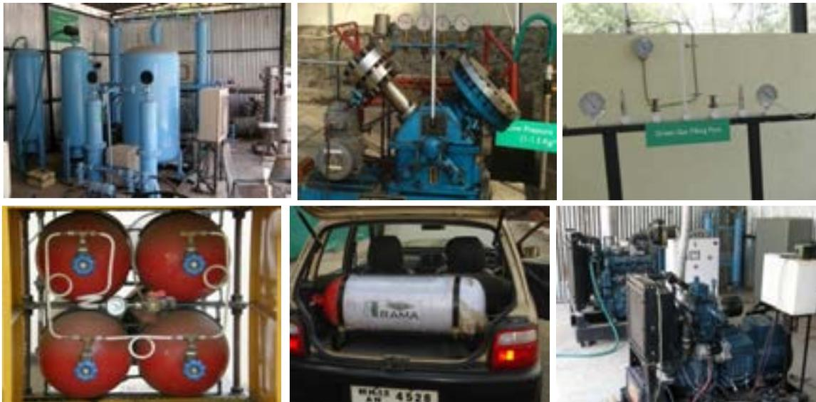
**EXPERIMENTAL SETUP FOR BIOGAS TO FUEL (SCRUBBER, COMPRESSOR, STORAGE, DISPENSING TO USE) AND BIOGAS TO POWER (GENSET)**
